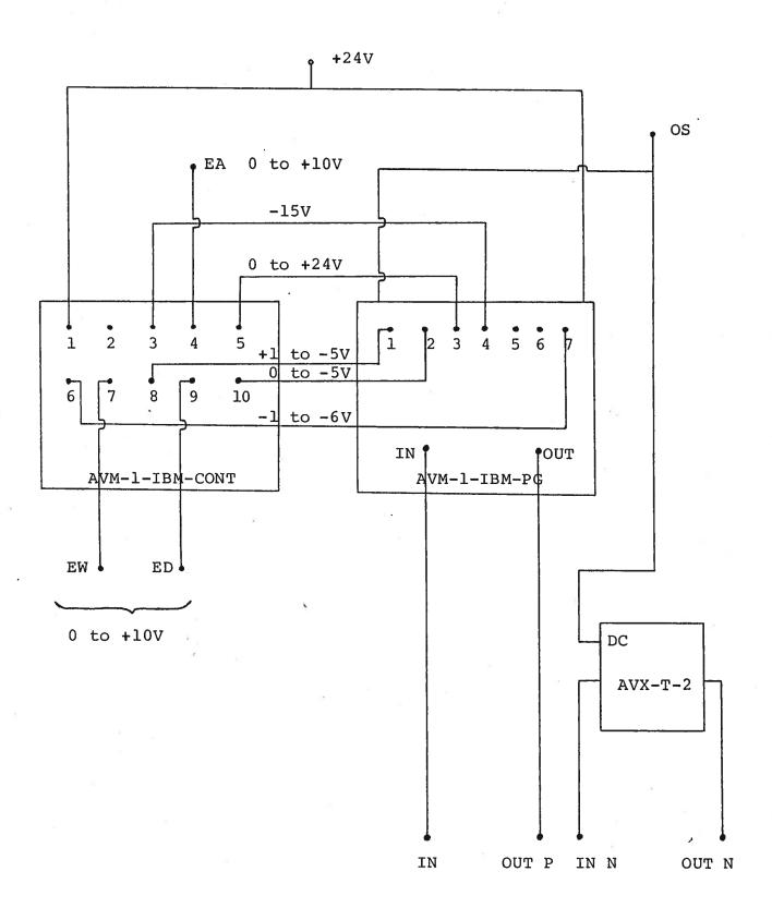
Fig. 2 AVM-1-IBM-1 BLOCK DIAGRAM
