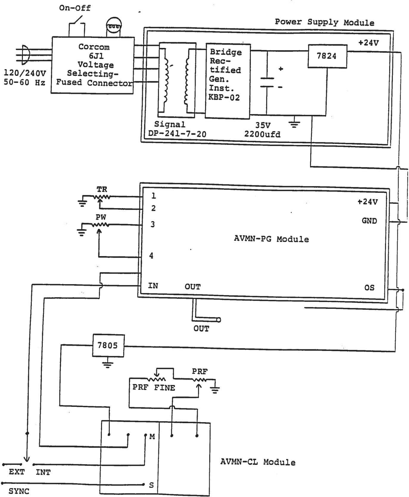
FIG 5: SYSTEM BLOCK DIAGRAM (WITH EA, EW, ED OPTIONS)
