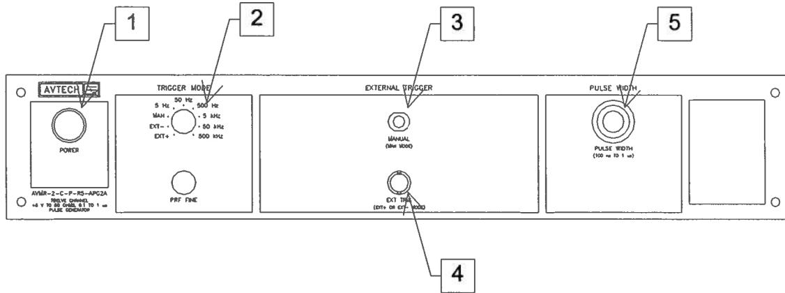
1. **POWER Switch.** The POWER push button switch applies AC prime power to the primaries of the transformer, turning the instrument on. The push button lamp (#382 type) is connected to the internal +15V DC supply.
