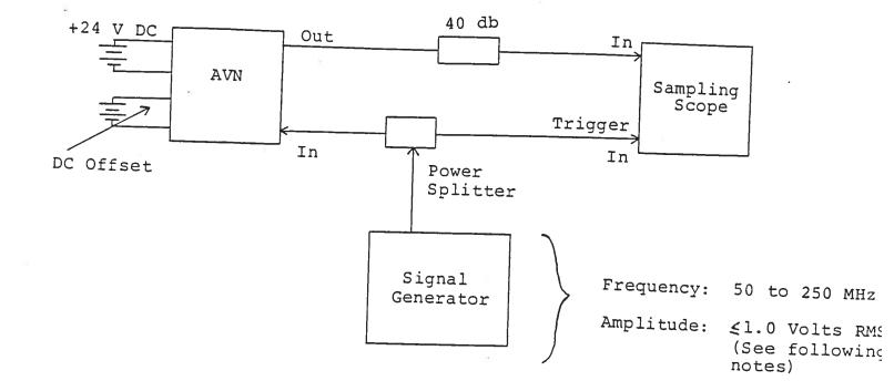
While increasing the signal generator output simultaneously insure that the AVN supply current does not exceed 0.45 Amps.
