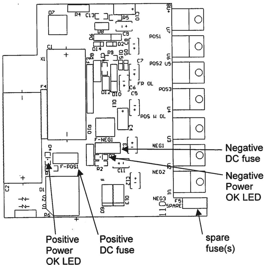
The positive fuse and one of the spare fuses on this circuit board are 1.5A slow-blow fuses, Littlefuse part number R45201.5. (This fuse can be ordered from Digikey, [www.digikey.com](http://www.digikey.com). The Digikey part number is F1344CT-ND). The negative fuse is a 0.5A slow-blow fuse (Littlefuse R452.500, Digikey part number F1341CT-ND).
