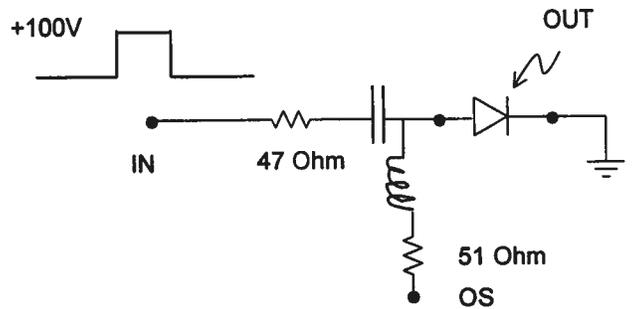
**FIG. 1C: AVO-2T-BEO2B3 Functional Equivalent Circuit**
