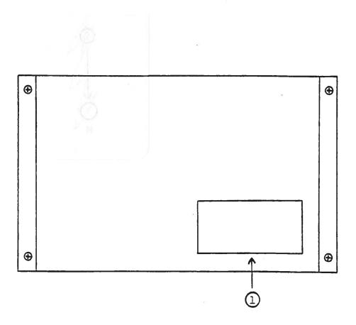
(1) <u>FUSED CONNECTOR, VOLTAGE SELECTOR</u>. The detachable power cord is connected at this point. In addition, the removable cord is adjusted to select the desired input operating voltage. The unit also contains the main power fuse (0.25 A SB).
