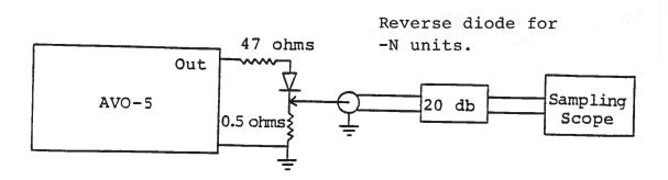
The output current may be observed by placing a 0.5 Ohm carbon composition resistor in series with the diode and placing a 50 Ohm cable across this resistor. With this arrangement, output current rise times of one nanosecond are possible.
