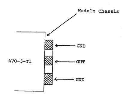
The diode load and series resistor (3.0 Ohm 1/4 W carbon composition resistor) should be connected between the OUT and GND terminals using very short leads ( $\leq 0.2$  cm). The voltage across the resistor-diode load may be monitored by connecting a length of 80 mil semi-rigid 50 Ohm cable as shown below:
