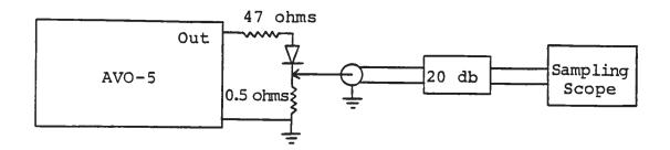
The output current may be observed by placing a 0.5 Ohm carbon composition resistor in series with the diode and placing a 50 Ohm cable across this resistor. With this arrangement, output current rise times of one nanosecond are possible.
