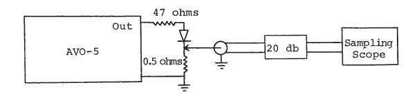
The output current may be observed by placing a 0.5 ohm carbon composition resistor in series with the diode and placing a 50 ohm cable across this resistor. With this arrangement, output current rise times of one nanosecond are possible.
