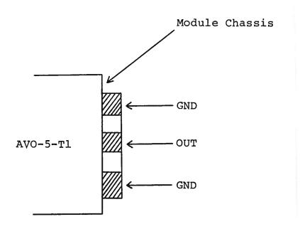
The diode load and series resistor (3.0 ohm 1/4 W carbon composition resistor) should be connected between the OUT and GND terminals using very short leads (< 0.2 cm). The voltage across the resistor-diode load may be monitored by connecting a length of 80 mil semi-rigid 50 ohm cable as shown below:
