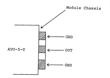
The diode load and series resistor (3.0 ohm 1/4 W carbon composition resistor) should be connected between the OUT and GND terminals using very short leads ( $\leq$  0.2 cm). The voltage across the resistor-diode load may be monitored by connecting a length of 80 mil semi-rigid 50 ohm cable as shown below:
