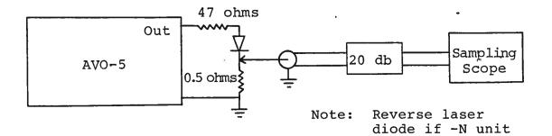
The output current may be observed by placing a 0.5 ohm carbon composition resistor in series with the diode and placing a 50 ohm cable across this resistor. With this arrangement, output current rise times of one nanosecond are possible.
