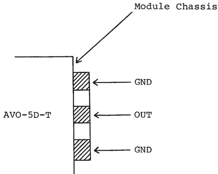
The diode load and series resistor (2.5 to 3.5 ohm 1/2 W carbon composition resistor) should be connected between the OUT and GND terminals using very short leads ( $\ll 0.5$  cm). The voltage across the resistor-diode load may be monitored by connecting a length of 80 mil semi-rigid 50 ohm cable as shown below:
