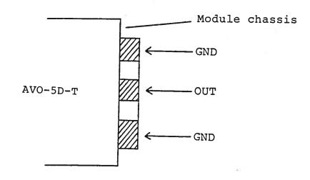
The diode load and series resistor (3 ohm 2 W carbon composition resistor) should be connected between the DUT and GND terminals using very short leads ( $\leq$  1.0 cm). The voltage across the resistor-diode load may be monitored by means of a high impedance scope probe.
