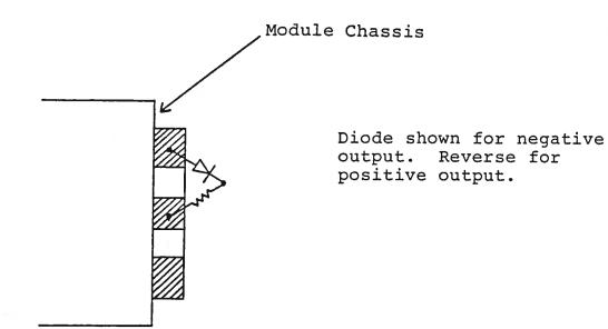
Take care to insure that during soldering the OUT conductor is not shorted to the chassis. Also, use minimal heat when soldering.
