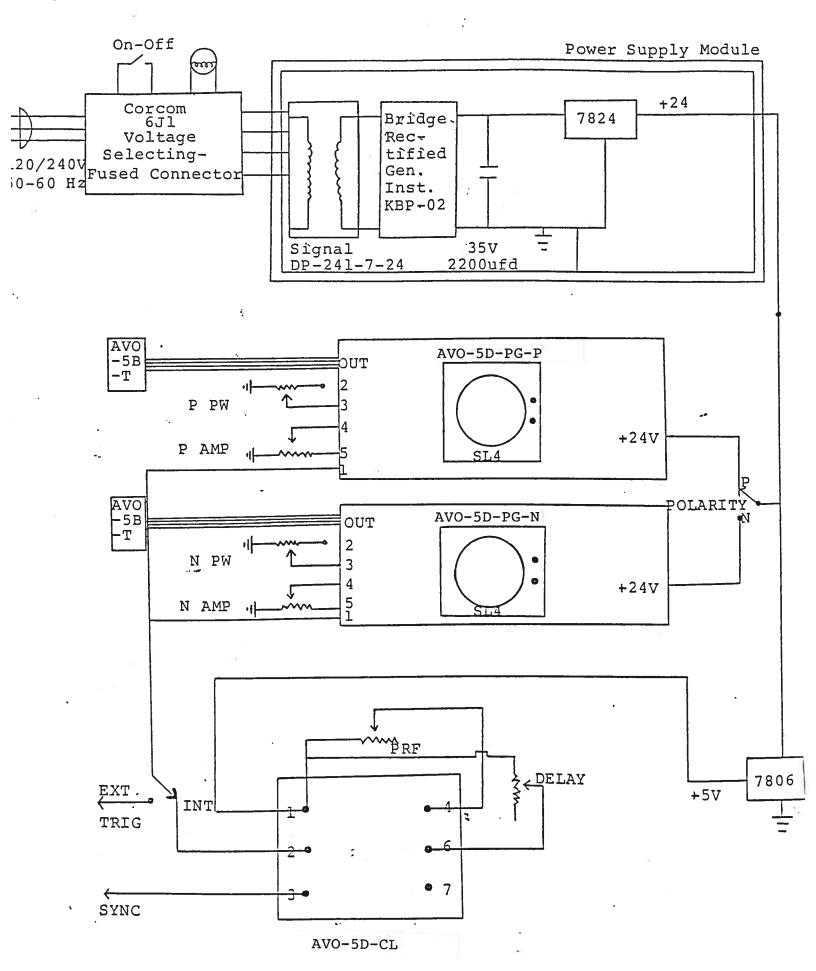
The AVD-5D-C-PN unit consists of the following basic modules:
