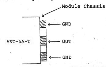
The diode load and series resistor (3.0 ohm  $\frac{1}{4}$  W carbon composition resistor) should be connected between the OUT and GND terminals using very short leads ( $\leq 0.2$  cm). The voltage across the resistor-diode load may be monitored by connecting a length of 80 mil semi-rigid 50 ohm cable as shown below:
