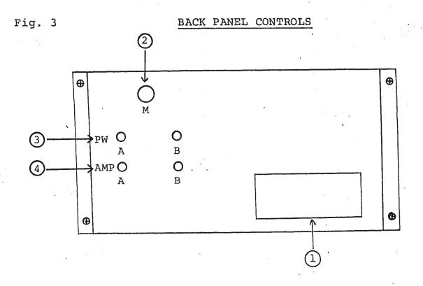
FUSED CONNECTOR, VOLTAGE SELECTOR. The detachable power cord is connected at this point. In addition, the removable cord is adjusted to select the desired input operating voltage. The unit also contains the main power fuse. 2 MONITOR Output (M). Output voltage (to fifty ohms) at this point ( $V_M$ ) can be related to AVO-5A-T output current ( $I_{OUT}$ ) as follows (option):
