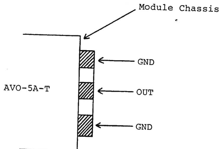
The diode load and series resistor (2.5 to 3.5 ohm 2 W carbon composition resistor) should be connected between the OUT and GND terminals using very short leads ( $\ll 0.5$  cm). The voltage across the resistor-diode load may be monitored by connecting a length of 80 mil semi-rigid 50 ohm cable as shown below:
