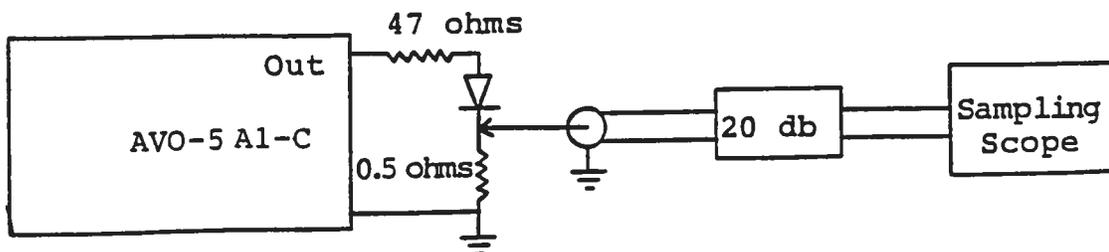
The output current may be observed by placing a 0.5 Ohm carbon composition resistor in series with the diode and placing a 50 Ohm cable across this resistor.
