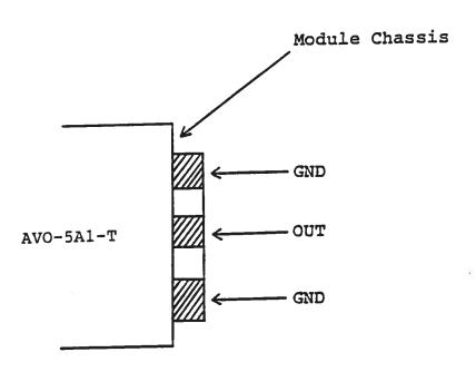
The diode load and series resistor (10 Ohm 1/4 W carbon composition resistor) should be connected between the OUT and GND terminals using very short leads (< 0.2 cm). The voltage across the resistor-diode load may be monitored by connecting a length of 80 mil semi-rigid 50 Ohm cable as shown below:
