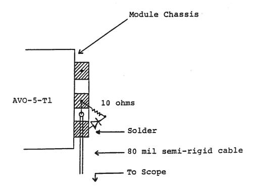
Take care to insure that during soldering the OUT conductor is not shorted to the chassis. Also, use minimal heat when soldering. The series resistor may be varied between about 7 to 15 Ohms with minimal waveform degradation.
