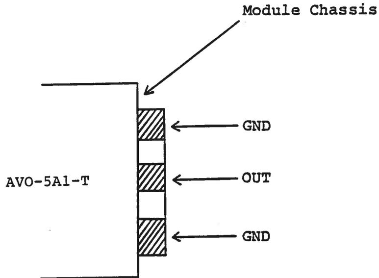
The diode load and series resistor (10 Ohm 1/4 W carbon composition resistor) should be connected between the OUT and GND terminals using very short leads (< 0.2 cm). The voltage across the resistor-diode load may be monitored by connecting a length of 80 mil semi-rigid 50 Ohm cable as shown below:
