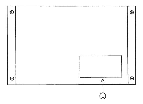
(1) <u>FUSED CONNECTOR, VOLTAGE SELECTOR</u>. The detachable power cord is connected at this point. In addition, the removable cord is adjusted to select the desired input operating voltage. The unit also contains the main power fuse.
