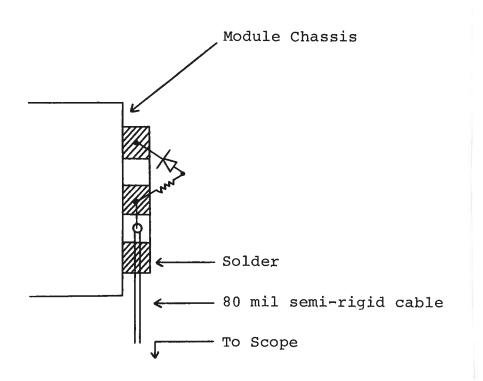
Take care to insure that during soldering the OUT conductor is not shorted to the chassis. Also, use minimal heat when soldering. The voltage may also be monitored using a high impedance scope probe.
