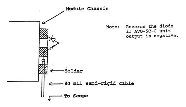
Take care to insure that during soldering the OUT conductor is not shorted to the chassis. Also, use minimal heat when soldering.
