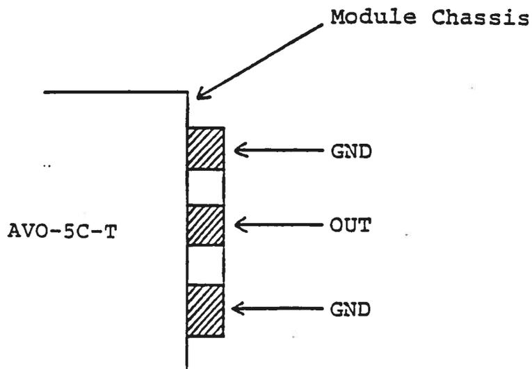
The diode load and series resistor (6 Ohm or 1.5 Ohm 1/2 W carbon composition resistor) should be connected between the OUT and GND terminals using very short leads ( $\leq 0.2$  cm). The voltage across the resistor-diode load may be monitored by connecting a length of 80 mil semi-rigid 50 Ohm cable as shown below:
