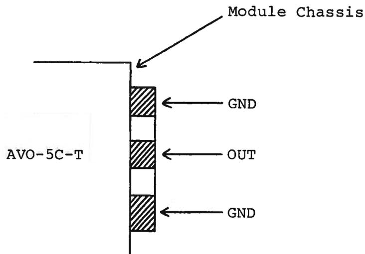
The diode load and series resistor (1.2 to 1.7 ohm 1/4 W carbon composition resistor) should be connected between the OUT and GND terminals using very short leads ( $\leq 0.2$  cm). The voltage across the resistor-diode load may be monitored by connecting a length of 80 mil semi-rigid 50 ohm cable as shown below:
