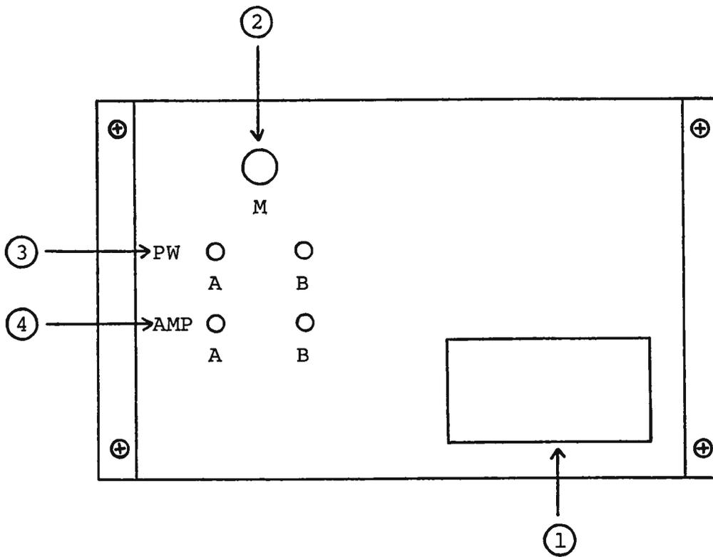
(1) FUSED CONNECTOR, VOLTAGE SELECTOR. The detachable power cord is connected at this point. In addition, the removable cord is adjusted to select the desired input operating voltage. The unit also contains the main power fuse.
