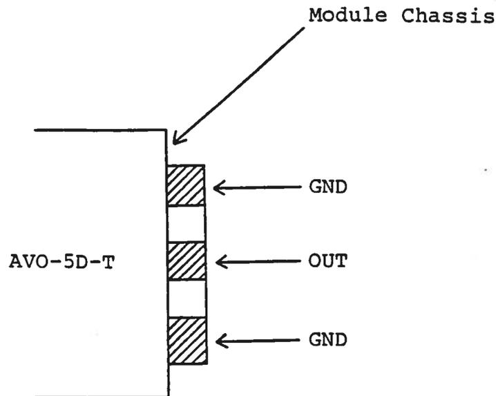
The diode load and series resistor (2.5 to 3.5 Ohm 1/2 W carbon composition resistor) should be connected between the OUT and GND terminals using very short leads ( $\leq 0.5$  cm). The voltage across the resistor-diode load may be monitored by connecting a length of 80 mil semi-rigid 50 Ohm cable as shown below:
