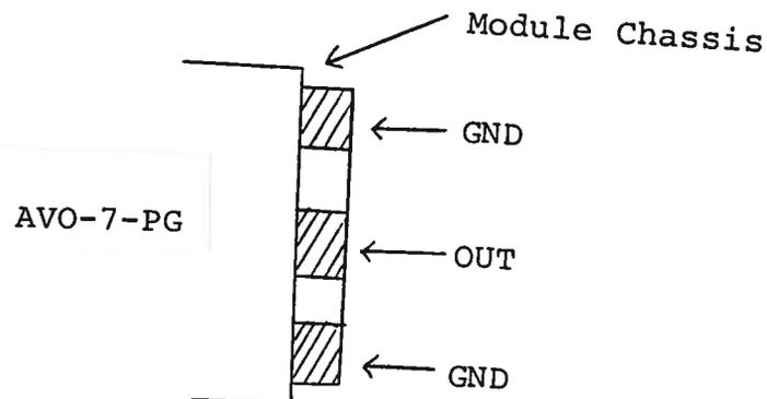
The load should be connected between the OUT and GND terminals using very short leads ( $\ll 0.5$  cm). The voltage across the load may be monitored by connecting a length of 80 mil semi-rigid 50 ohm cable as shown below (or by means of a high impedance scope probe):
