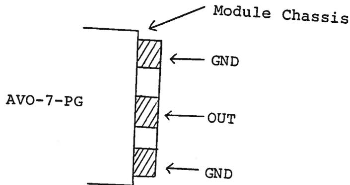
The load should be connected between the OUT and GND terminals using very short leads ( $\ll 2.0$  cm). The voltage across the load may be monitored by connecting a length of 80 mil semi-rigid 50 ohm cable as shown below (or by means of a high impedance scope probe):
