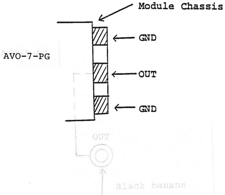
The load should be connected between the OUT and GND terminals using very short leads ( $\ll 1.0''$ ). Leads of up to 12" may be used but heavy wire (eg. #12) twisted pair or 1/2" wide strips of copper plate should be used in order to reduce the deterioration of rise time.
