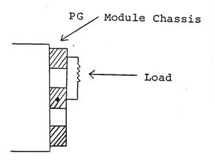
Take care to insure that during soldering the OUT conductor is not shorted to the chassis. Also, use minimal heat when soldering. A BNC output connector (in parallel with the microstrip output) is also provided.
