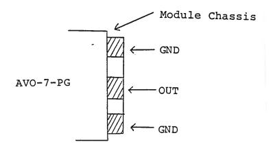
The load should be connected between the OUT and GND terminals. The voltage across the load may be monitored by means of a high impedance scope probe.
