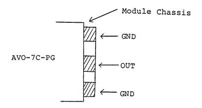
The load should be connected between the DUT and GND terminals using very short leads (<0.5 cm). The voltage across the load may be monitored by connecting a length of 80 mil semi-rigid 50 ohm cable as shown below (or by means of a high impedance scope probe):
