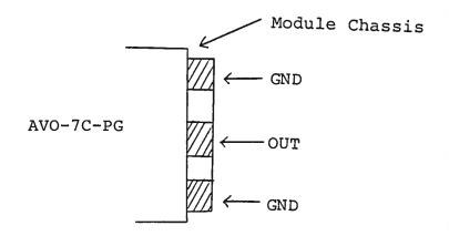
The load should be connected between the OUT and GND terminals using very short leads ( $\langle 0.5 \text{ cm} \rangle$ ). The voltage across the load may be monitored by connecting a length of 80 mil semi-rigid 50 ohm cable as shown below (or by means of a high impedance scope probe):
