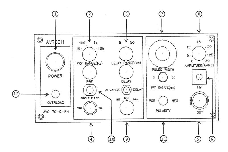
(1) ON-OFF Switch. Applies basic prime power to all stages.
