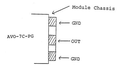
The load should be connected between the OUT and GND terminals using very short leads ( $\leq 0.5 \text{ cm}$ ). The voltage across the load may be monitored by connecting a length of 80 mil semi-rigid 50 ohm cable as shown below (or by means of a high impedance scope probe):
