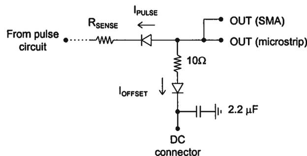
(Note that these drawings illustrate the  $R_{\text{SENSE}}$  resistor and the  $10\Omega$  resistor used to generate the monitor output.)
