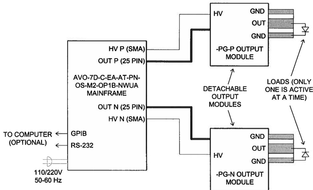
The loads can be connected (soldered) to a microstrip transmission line that protrudes from the output module, or they can be connected via a SMA connector located directly
