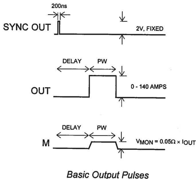
The delay, pulse width, and frequency (when in the internal mode), of the OUT pulse can be varied with front panel controls or via the GPIB or RS-232 computer interfaces.
