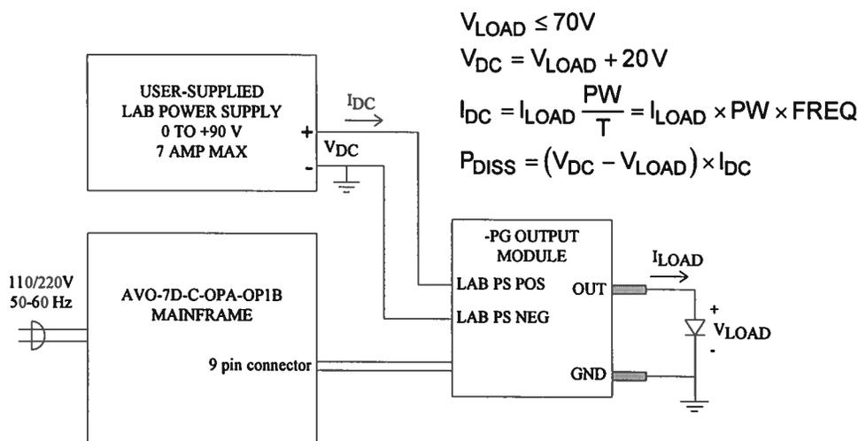
The AVO-7D-C-OPA-OP1B-P includes provision for water-cooling, which should be used when the power dissipated in the output module ( $P_{DISS}$ ) exceeds 30 Watts.
