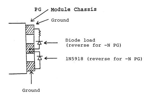
Take care to insure that during soldering the OUT conductor is not shorted to the chassis. Also, use minimal heat when soldering.
