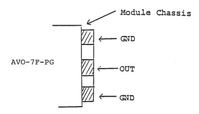
The load should be connected between the OUT and GND terminals using very short leads (≤ 1.0 cm). The diode current may be monitored using a current probe or by placing a fractional Ohm resistor (eg. 0.1 Ohm) in series with the diode to ground and monitoring the voltage across the resistor. A fast diode (eg. 1N5819) should be placed across the laser diode load to protect against reverse potentials.
