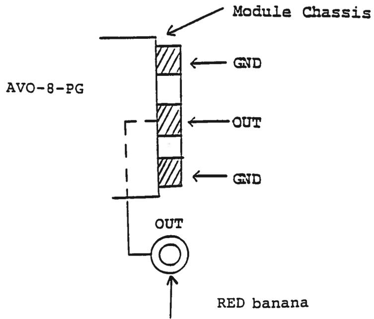
The load should be connected between the OUT and GND terminals using very short leads ( $\leq 2.0$  cm).
