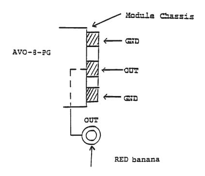
The load should be connected between the OUT and GND terminals using very short leads (≤ 2.0 cm).
