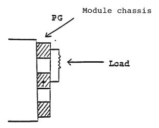
Take care to insure that during soldering the OUT conductor is not shorted to the chassis. Also, use minimal heat when soldering.
