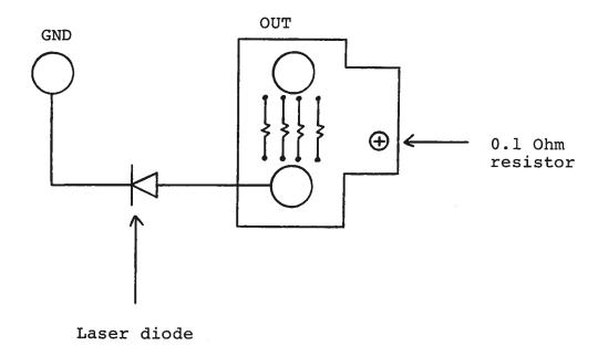
Note that the resistor module is suitable only for low duty cycle operation (eg. 1%). For high duty cycle operation, it should be replaced by a high power model.
