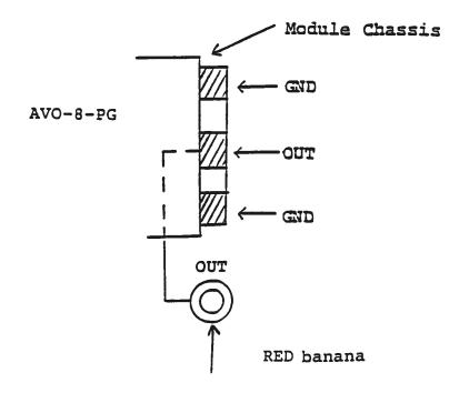
The load should be connected between the OUT and GND terminals using very short leads ( $\leq$  2.0 cm).
