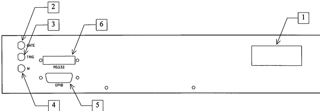
1. **AC POWER INPUT.** A three-pronged recessed male connector is provided on the back panel for AC power connection to the instrument. Also contained in this assembly is a 1.0A slow blow fuse and a removable card that can be removed and repositioned to switch between 120V AC in and 240V AC in.
