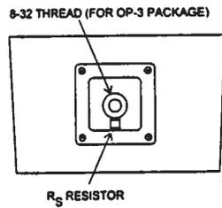
Fig. 4 - AVX-S3 input assembly (for OP-3 package)
