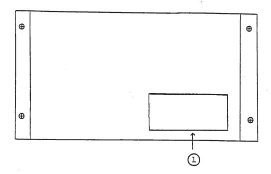
(1) FUSED CONNECTOR, VOLTAGE SELECTOR. The detachable power cord is connected at this point. In addition, the removable cord is adjusted to select the desired input operating voltage. The unit also contains the main power fuse (0.5 Amp SB).
