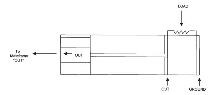
Note that the load should be greater than 0.3 Ohms.
