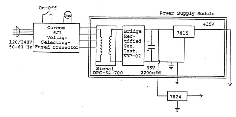
FIG. 5: AVP-2S-PN-EA-EW-EO-C BLOCK DIAGRAM
