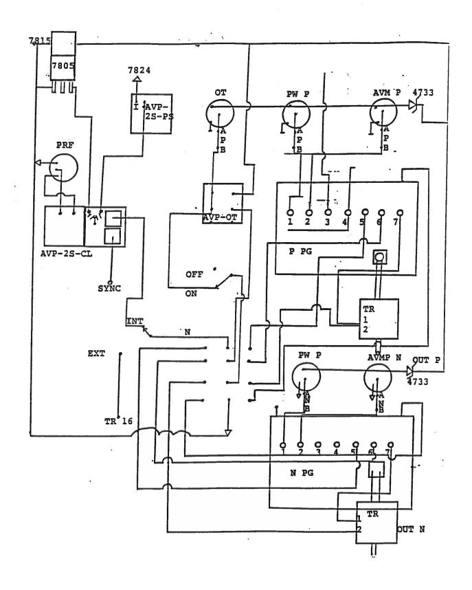
FIG. 6: AVP-2S-C-PN BLOCK DIAGRAM
