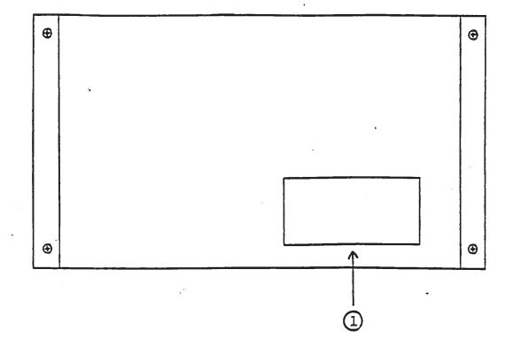
(1) <u>FUSED CONNECTOR, VOLTAGE SELECTOR</u>. The detachable power cord is connected at this point. In addition, the removable cord is adjusted to select the desired input operating voltage. The unit also contains the main power fuse (0.25 A SB).
