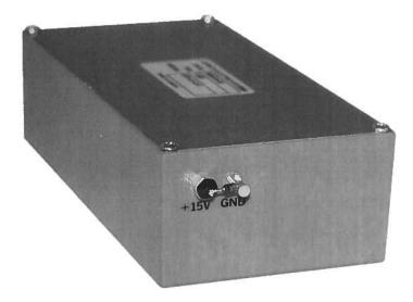
The +15V input terminal is protected with a 1N4746A Zener diode, which will fail as a short if an excessive positive voltage (> 18V), or a negative voltage, is applied to the terminal.
