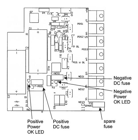
The spare fuse may be used to replace one of the other fuses, if required.
