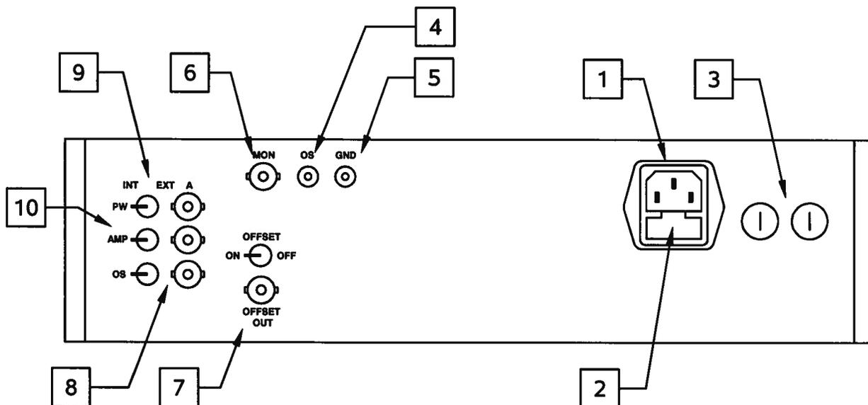
1. **AC POWER INPUT.** An IEC-320 C14 three-pronged recessed male socket is provided on the back panel for AC power connection to the instrument. One end of the detachable power cord that is supplied with the instrument plugs into this socket.
