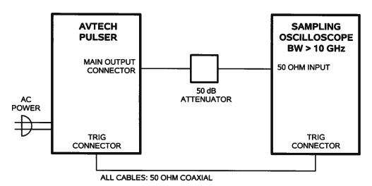
The attenuators are required to prevent damage to the sampling oscilloscope. A 50 dB attenuator with sufficient voltage rating should be used on the main output.
