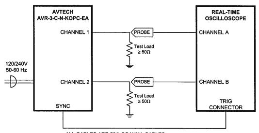
ALL CABLES ARE  $50\Omega$  COAXIAL CABLES.
