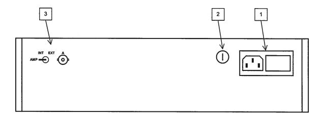
AC POWER INPUT. A three-pronged recessed male connector is provided on the back panel for AC power connection to the instrument. Also contained in this assembly is a slow blow fuse and a removable card that can be removed and repositioned to switch between 120V AC in and 240V AC in.
