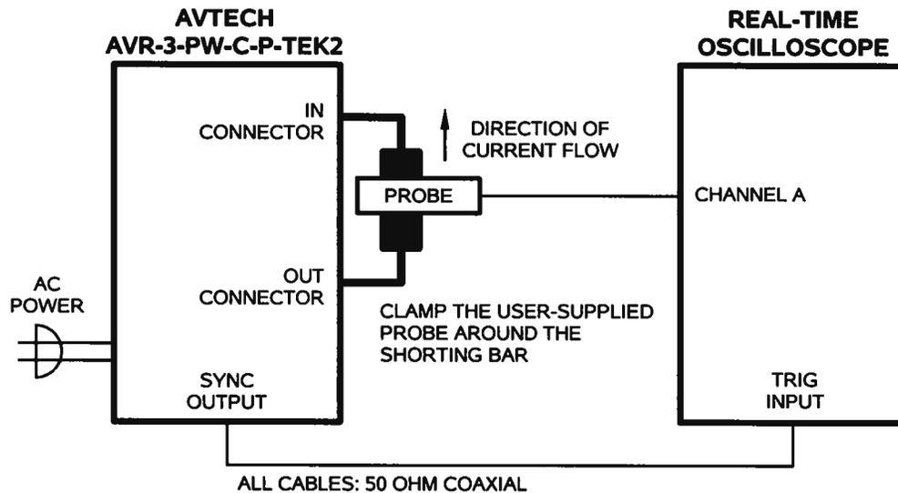
For other applications, the OUT terminal may be used to pulse a user-supplied 50 Ohm load, if desired. In this case, the shorting bar and the "IN" terminal are not used.
