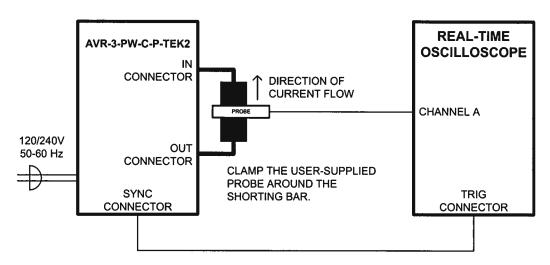
For other applications, the OUT terminal may be used to pulse a user-supplied 50 Ohm load, if desired. In this case, the shorting bar and the "IN" terminal are not used.
